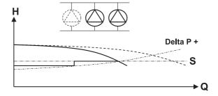
Figure 12: 2 pump operation
