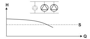
Figure 9: 2 main pumps operation
