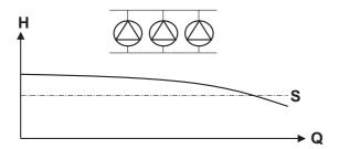
Figure 6: 3 pumps in operation
