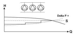
Figure 13: 3 pump operation
