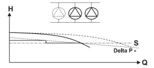
Figure 16: 2 pump operation
