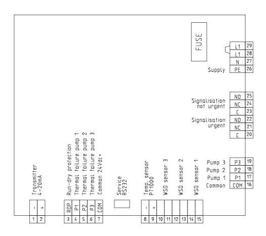
Figure 20: Electrical connections DP-Control II
