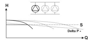
Figure 15: 1 pump operation
