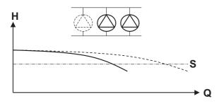
Figure 5: 2 pumps in operation
